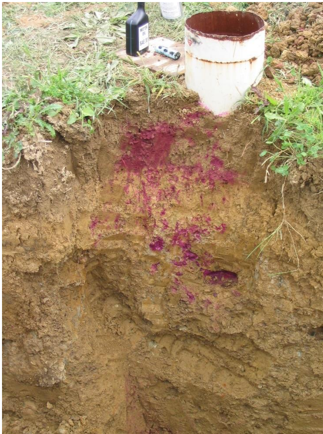
Plate D-2. Soil pit cut back to bucket containing dye to visualize transport of dye in the soil.
