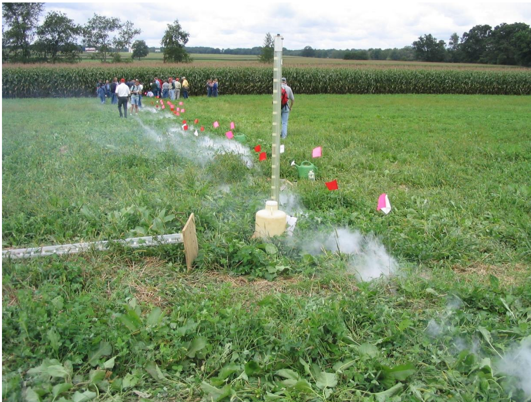
Plate D-4. Smoke from tile lines at the surface of a hay field.
