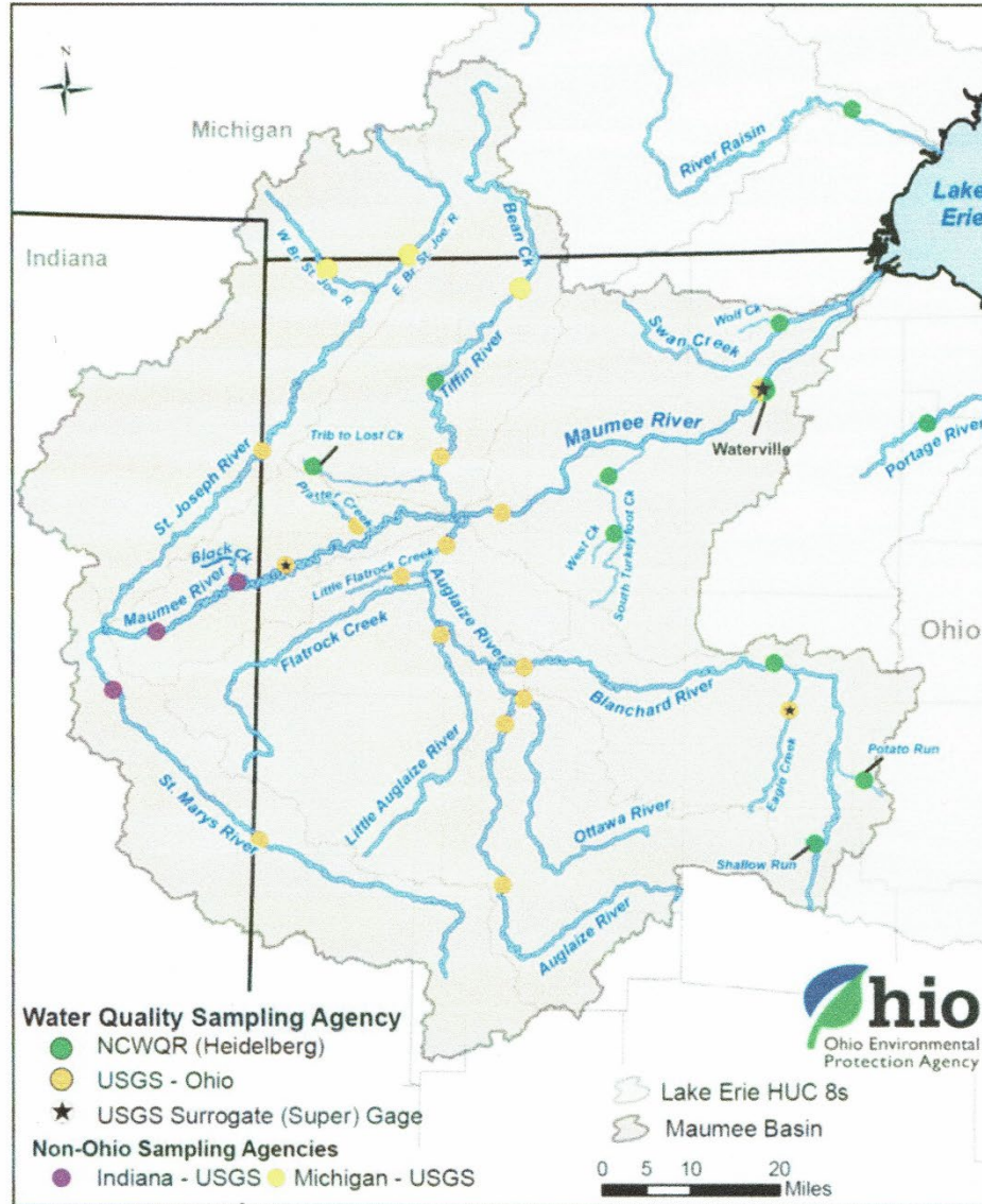
Figure 28. Network of continuous water quality monitoring stations throughout the Maumeé watershed at USGS streamflow gages. The various water quality sampling agencies are noted.
